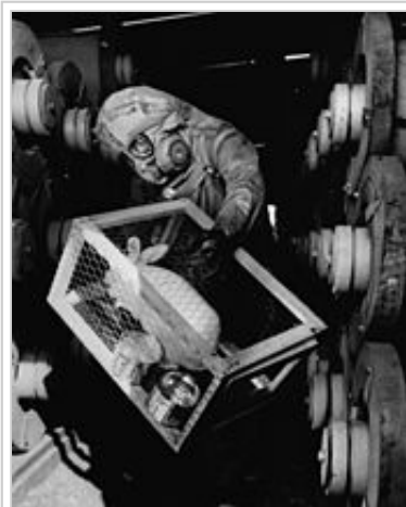
Rabbit used to check for leaks at sarin production plant, Rocky Mountain Arsenal (1970)
