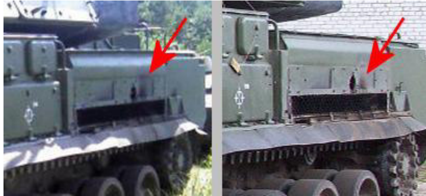
Buk 332 – Soot above the exhaust on Buk 332– details of photos 61 62
