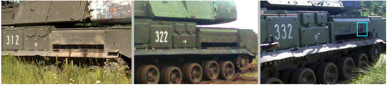
Soot deposits or oil stains at Buk 312, Buk 322 and Buk 332 – Details of photos 58 59 60
